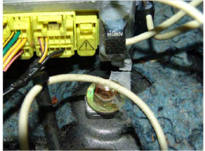
Figure 17. Fractured Mounting Flange to Module (Courtesy of Exponent 2011, Figure 23 )
