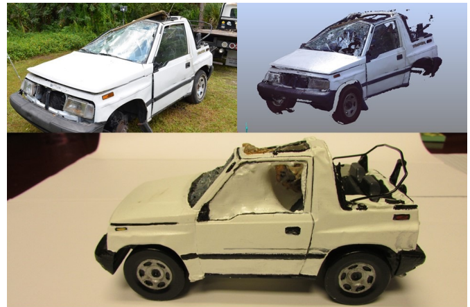
Photo 4 - Upper Left: Subject Vehicle, Upper Right: Vehicle Scan, Lower: 3D Printed Model
