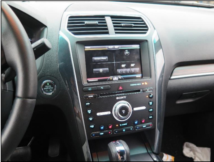
Figure 32. 2016 Ford Explorer: MyFord Touch, Sync Generation 2 Module
