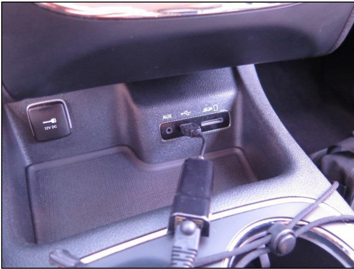
Figure 26. Logical Data Acquisition from the Dodge Durango
