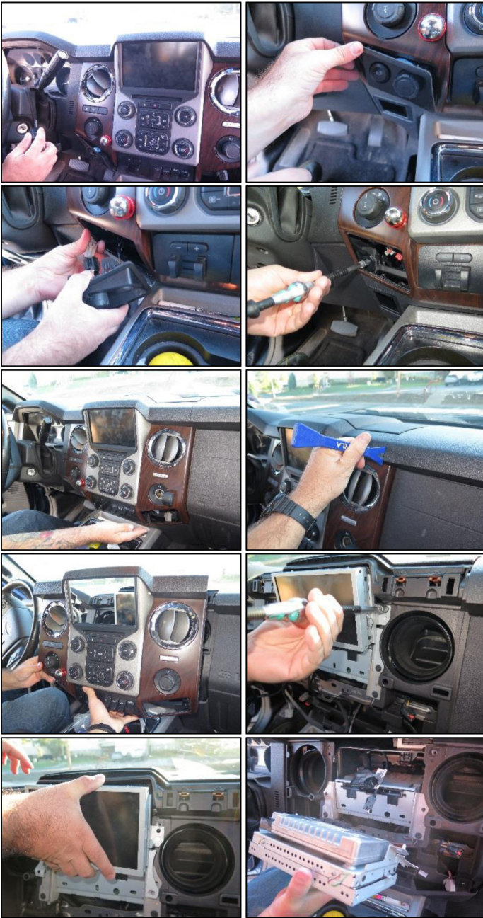
Figure 37. Physical Data Acquisition from the Ford F-350, Part 1
