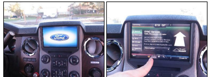
Figure 4. 2015 Ford F-350: MyFord Touch – Ford Sync, Generation 2 Module
