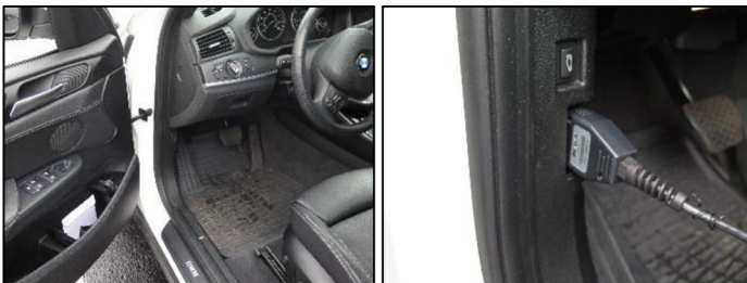
Figure 23. Logical Data Acquisition from the BMW X3 using OBD Port
