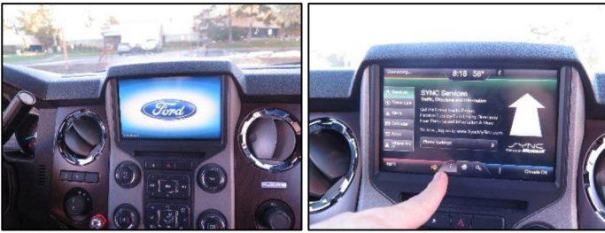
Figure 36. 2013 Ford F-150: MyFord Touch, Ford Sync, Generation 2 HMI
