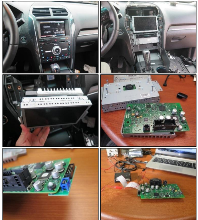
Figure 1. Sample Physical Acquisition 2016 Ford Explorer: Ford Sync, Generation 2 Module
