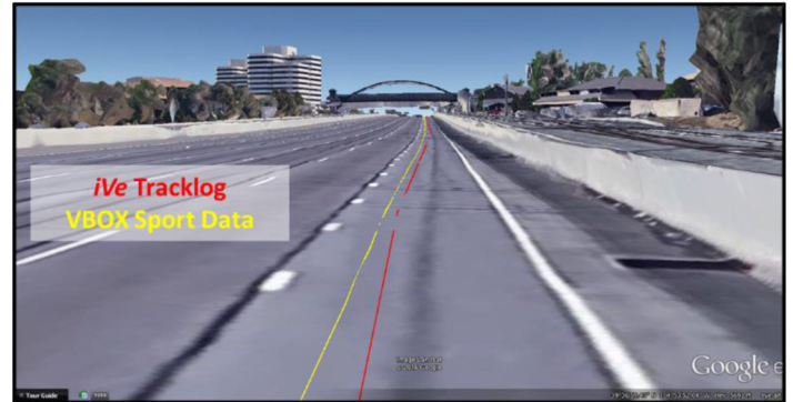
Figure 14. Comparison of Testing to GPS Data Vehicle Paths
