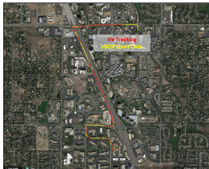
Figure 11. Case Study: Vehicle Tracklog Data Versus VBOX Sport Data
