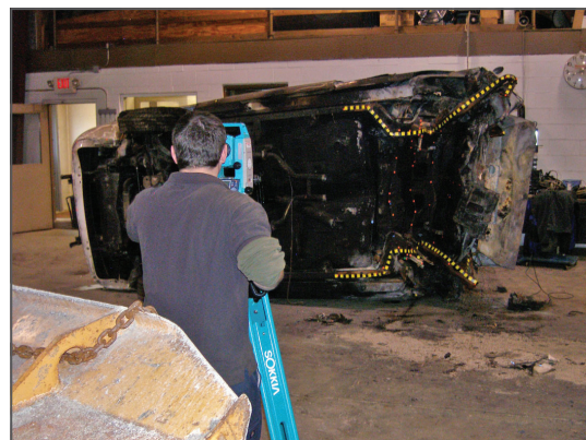
Figure 3 - Total station survey method: Accident Vehicle
