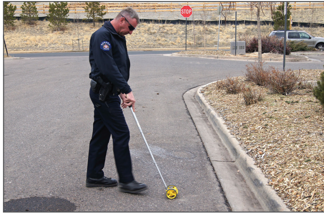
Figure 1 - Baseline Survey measurements using a roll-a-meter
