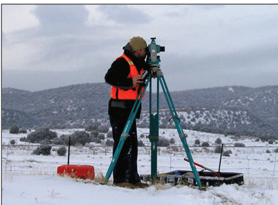
Figure 2 - Total station survey method: Accident Scene
