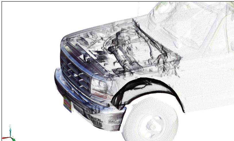
Figure 11 - 3D scan data with vehicle components visible
