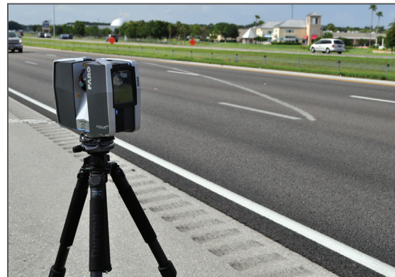
Figure 4 - 3D Laser Scanner: FARO Focus 3D
