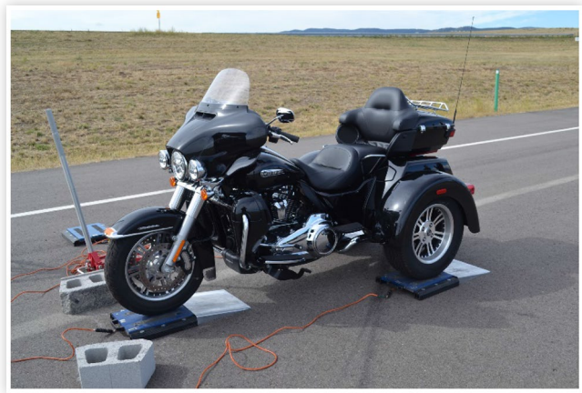
FIGURE 4 Motorcycle #1 being weighed with the front end elevated.
