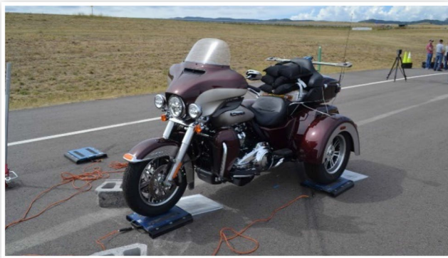
FIGURE 7 Motorcycle #2 with Ballast and Instrumentation
