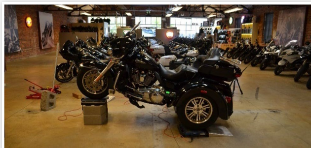
FIGURE 5 Motorcycle #1 being again weighed with the front end elevated.
