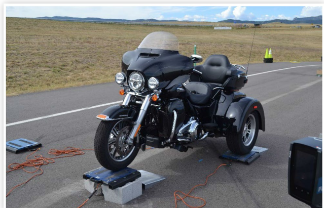
FIGURE 4 Motorcycle #1 being weighed with the front end elevated.
