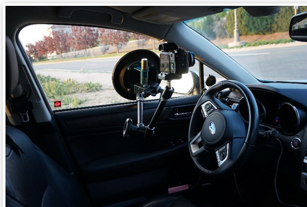
FIGURE 4 Camera setup in vehicle to capture driver's view
