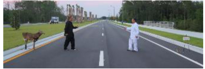
Figure 3. Photograph showing the five targets utilized in the experimentation (Deer, black clothing, white clothing, small rabbit, and license plate)
