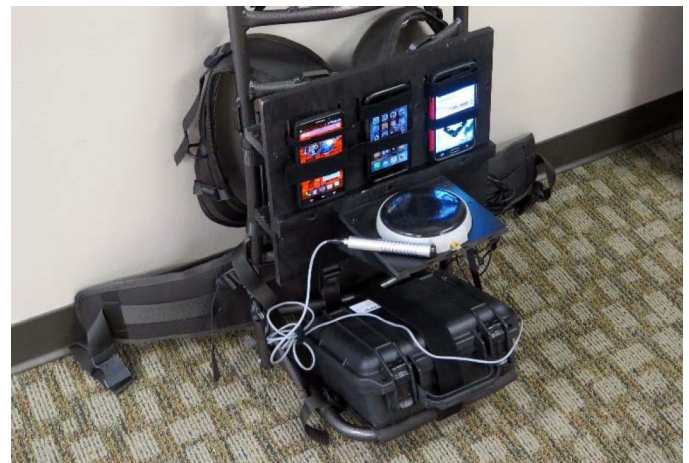
Figure 1. Backpack rig with smart phones and VBOX unit
