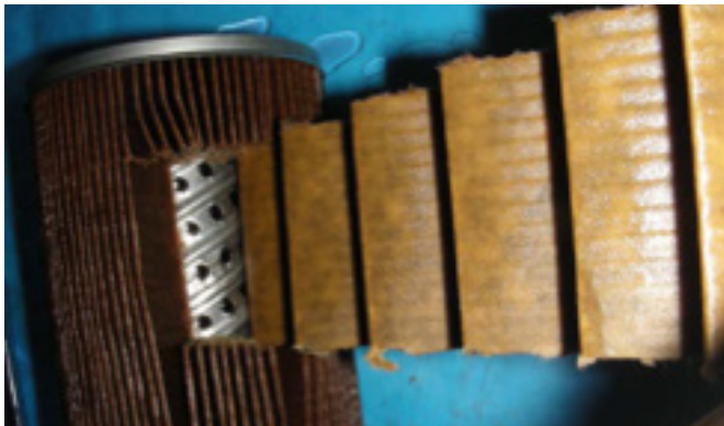
Figure 15 - Secondary fuel filter section removed for examination.
