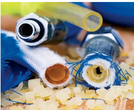
Figure 10 - TPU scuba air hoses at various stages of degradation.
