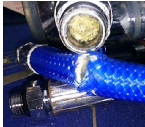
Figure 11 - Severely degraded TPU hose clogging air hose.
