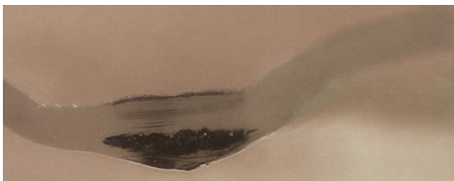
Figure 7 - Cross section of black particle and liner showing that it was embedded in the bulk of the polyethylene liner.
