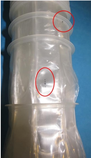
Figure 2 - Black contamination on the walls of the liners.
