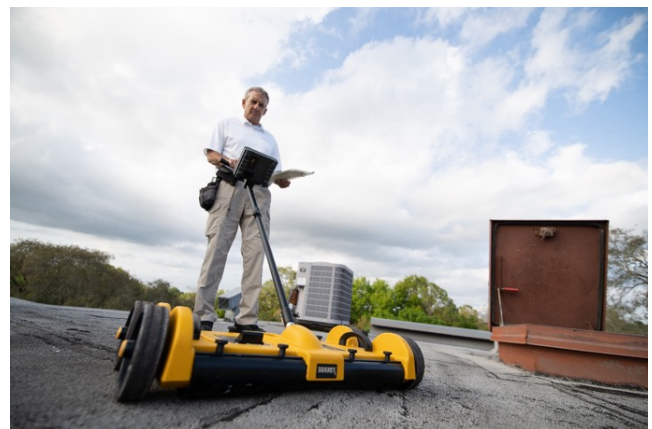
Figure 4 - Evaluating roofing materials for moisture.
