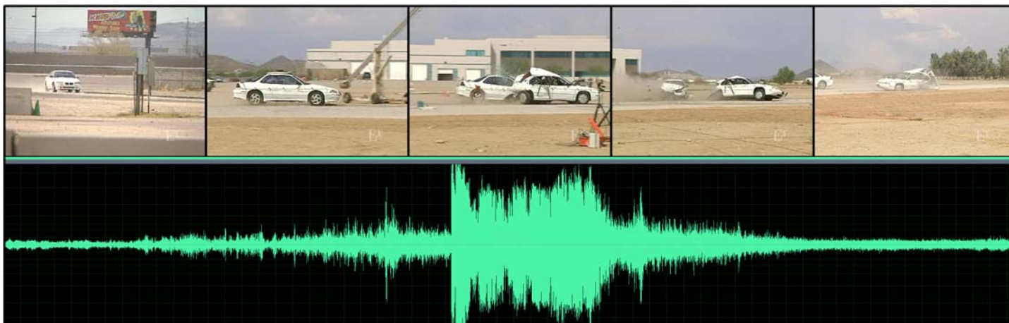
Figure 5 - Waveform showing increase in sound level at impact
