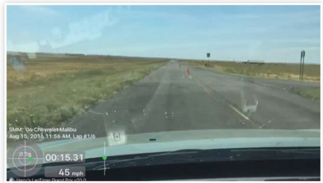
FIGURE 22 - Video Image from Harry's Lap Timer™ overlaid with data
