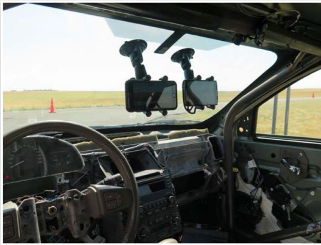
FIGURE 21 Droid and iPhone mounted to the windshield
