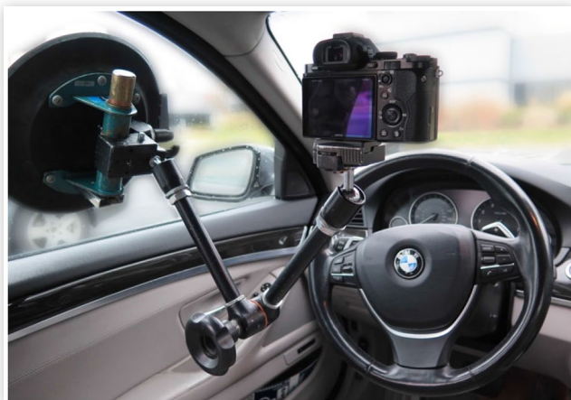
FIGURE 11 Setup of the nighttime photography equipment
