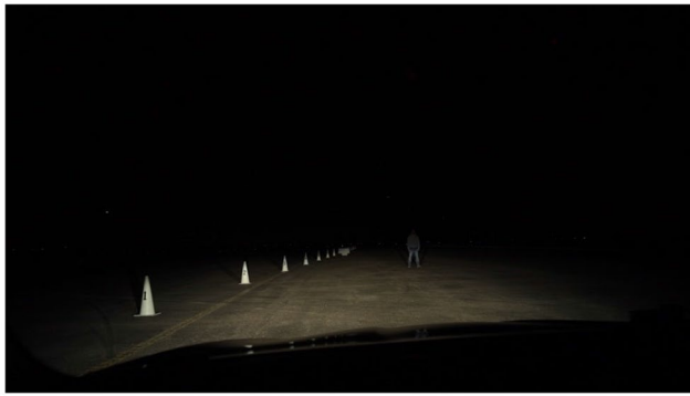
FIGURE 13 Photograph documenting contribution from full moon (2:30), pedestrian at 75 feet
