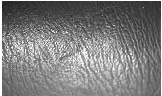
Figure 19. A fabric mark consisting of light diagonal abrasions was left on the rear fixed window lower plastic trim as a result of the ejection of ATD 3L in the Expedition rollover test.
