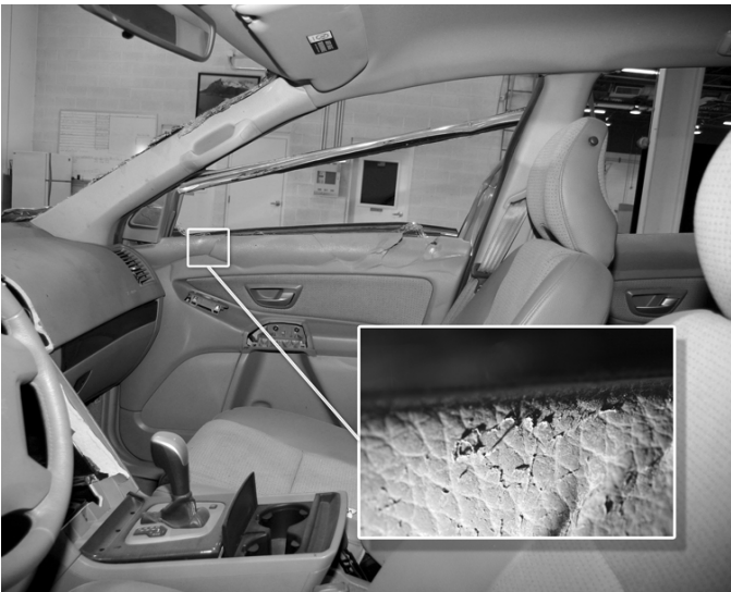
Figure 16. A scuff mark with upward and outboard smearing of the plastic was left on the beltline as a result of the ejection of ATD 1R in the Volvo rollover test.
