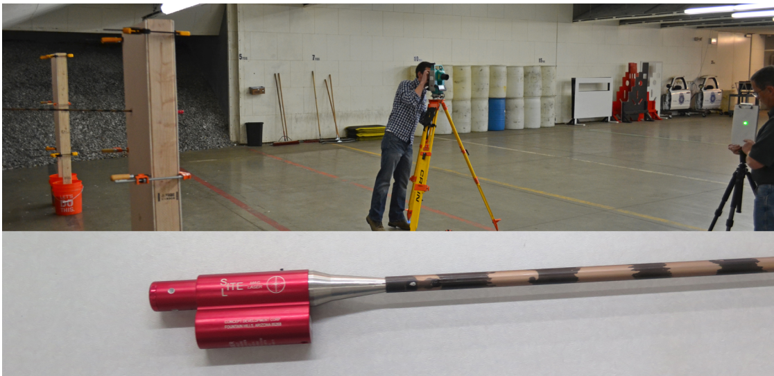
FIGURE 6: Laser trajectory mapping was completed using a boresight and mapped using a total station as shown above.
