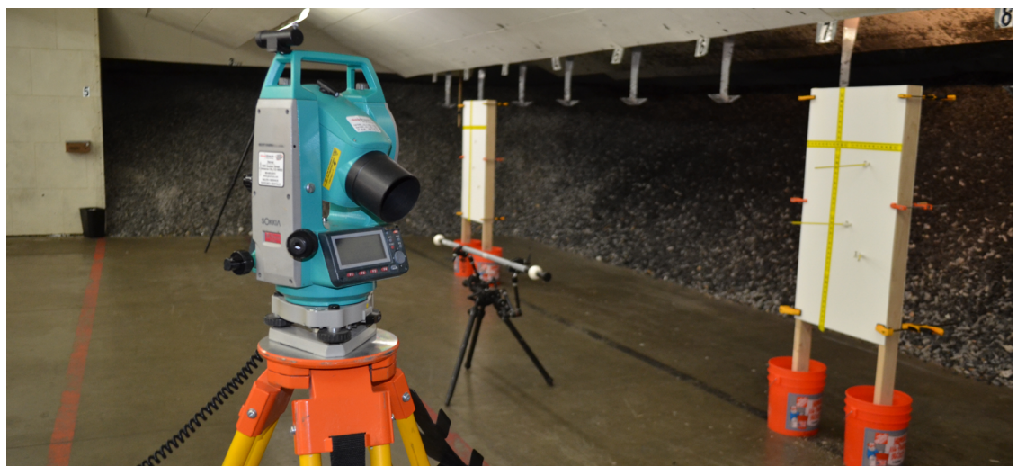
FIGURE 5: Total station mapping was completed using a Sokkia set 530R3 reflectorless total station (Method 2).
