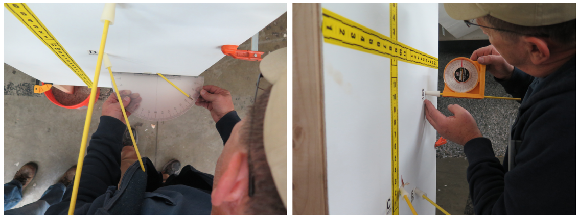
FIGURE 4: Hand measurements were made using a zero-edge protractor and inclinometer (Method 1).
