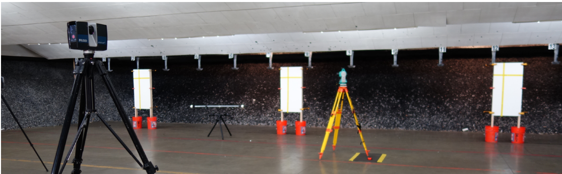
FIGURE 2: The testing setup had three targets and was documented using a total station and 3D laser scanning.
