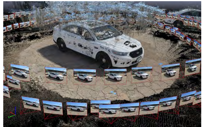
Figure 7. Photogrammetry point cloud solution with camera locations and photographs displayed. Canon PowerShot G16, 159 photographs processed in Pix4Dmapper.
