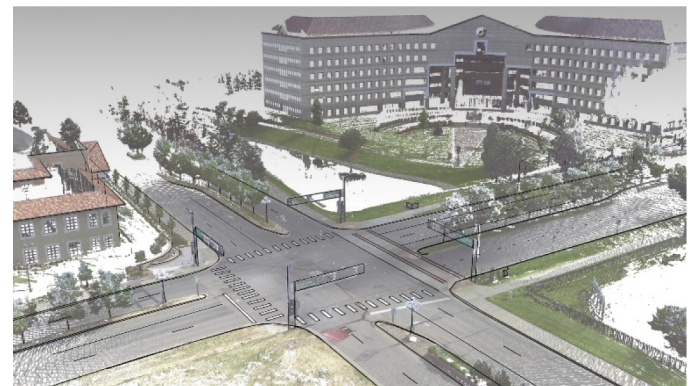
Figure 4. LiDAR data of the scene mapping. The color point cloud data is from the 3D laser scanner and black line work is from LiDAR data collected with the total station.
