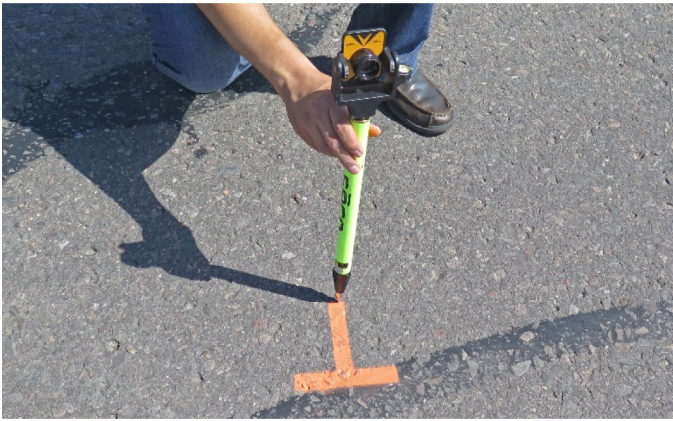
Figure 5. Orange spray chalk, representing evidence on the roadway surface, being recorded with a total station.
