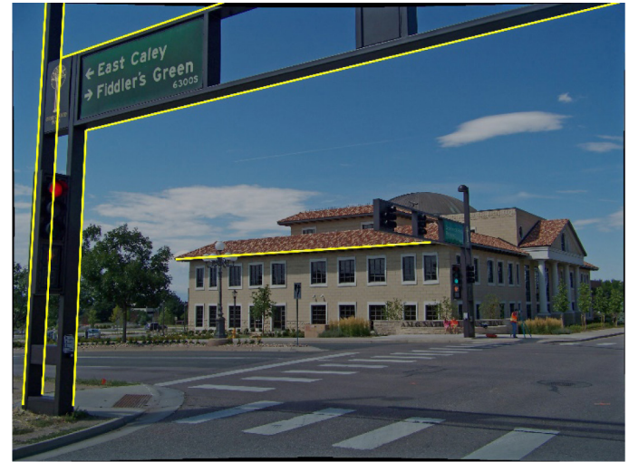
Figure 9. Photograph showing example of several linear objects used for removing lens distortion. This photograph was taken with the Kodak Z8612.
