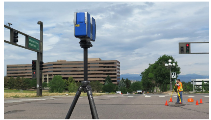
Figure 3. Test study site being mapped with a 3D laser scanner and a reflectorless total station.
