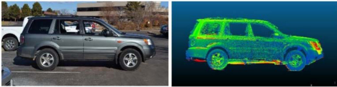
Figure 16. Photograph and Computer Model of Vehicle
