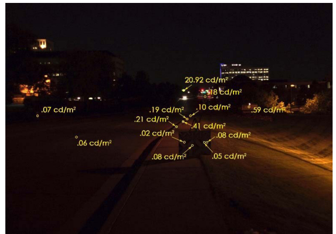
Figure 7. Nighttime Image with Luminance Measurements
