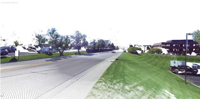
Figure 13. Scan Data of Environment Geometry
