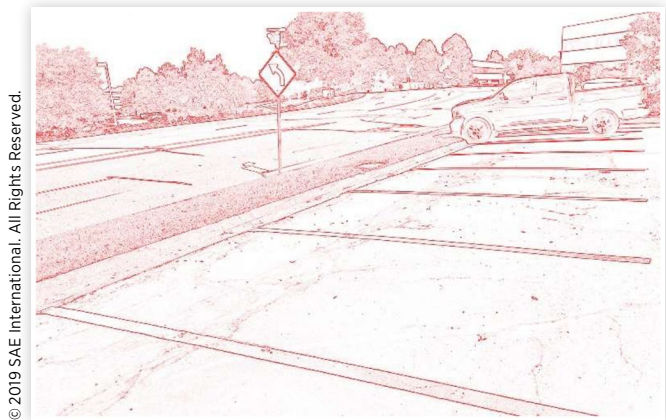
FIGURE 7 FoV determination: The resulting red outline photograph and live view alignment, with the photo FoV solution visible in the application interface.
