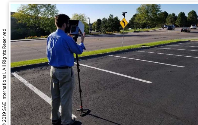
FIGURE 5 FoV determination: Solving for camera field-of-view in a nearby parking lot prior to visiting incident site.
