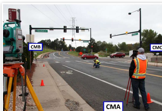
FIGURE 12 Placing tape at testing site, with 3 tablets positioned to solve for each camera as labeled: CMA, CMB, and CMC.
