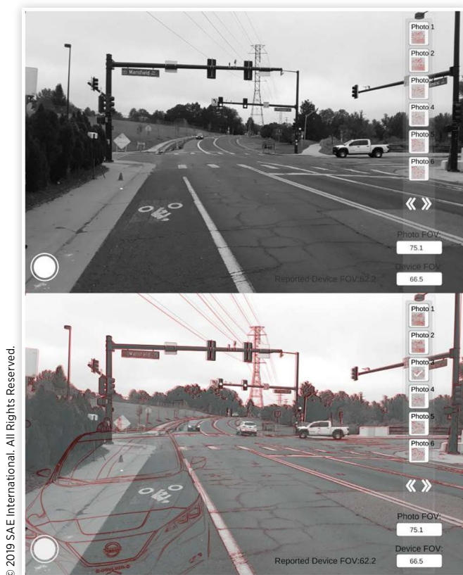
FIGURE 9 Application interface showing camera live view (Top) and red outlined photograph overlay aligned on top of live view (Bottom).
