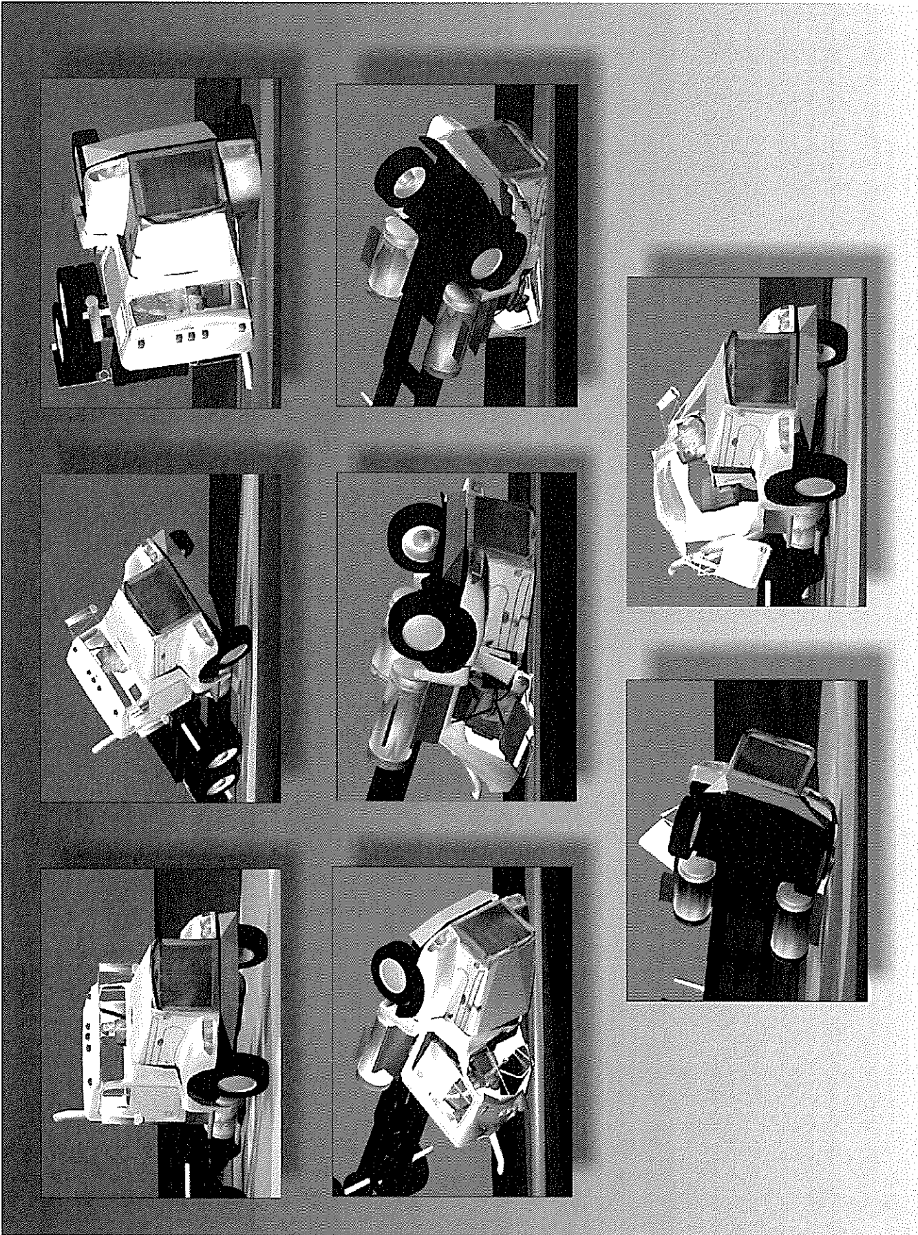
Figure 10. Analysis of Crush Sequence (Solid Model)
