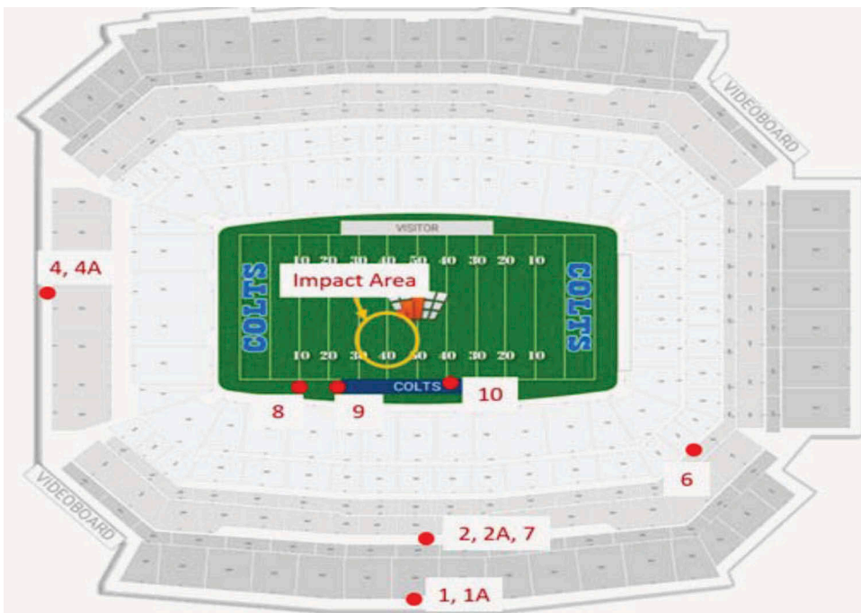
Figure 3. Location of cameras used for filming each impact event. camera locations were numbered, and cameras designated with an 'A' indicate a second camera at a higher frame rate at that location.
