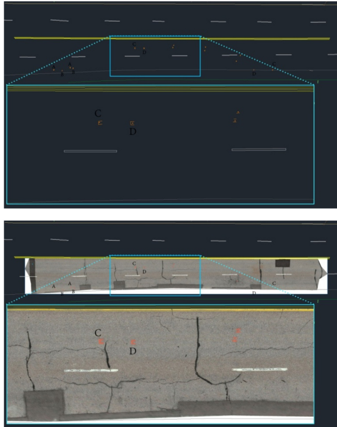
Figure 12. Image showing surveyed spray paint (top) and camera projected paint (bottom) marked with letters
