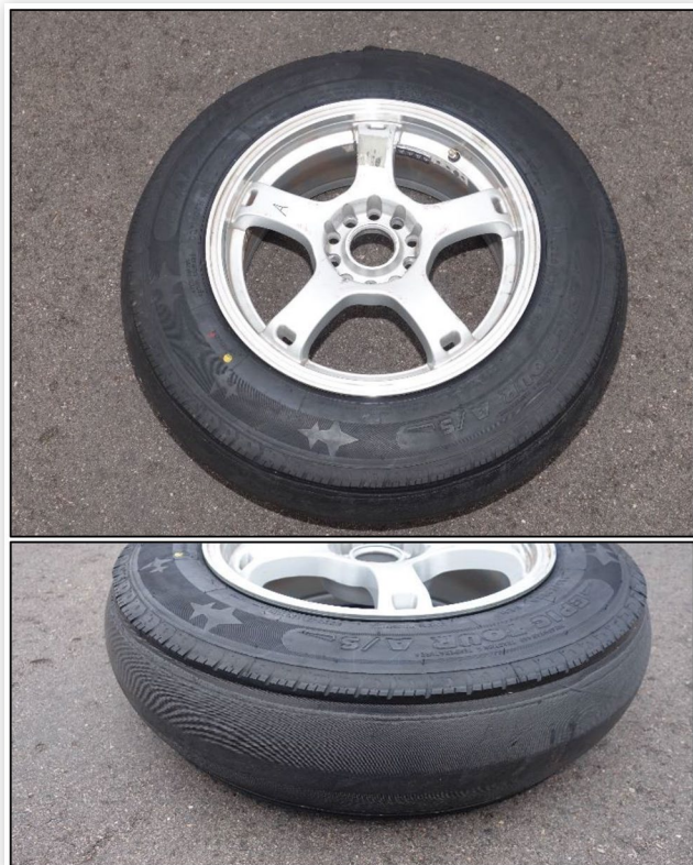
FIGURE 6 Tire with tread and top belt removed.
