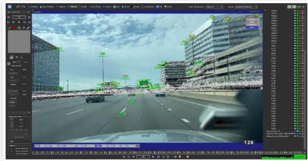
FIGURE 10 Video tracking solution shown within 3DS Max with LiDAR point cloud environment overlaid on the video.
