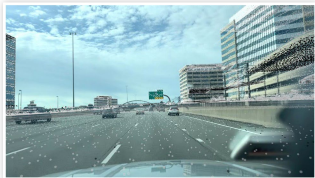
FIGURE 10 Video tracking solution shown within 3DS Max with LiDAR point cloud environment overlaid on the video.
