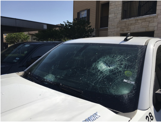
Figure 2 - Hail damage (Source: NOAA Damage Assessment Toolkit ( https://services.dat.noaa.gov/arcgis/rest/services/nws_damageassessmenttoolkit/DamageViewer/FeatureServer/0/1384003/attachments/837675 )).
