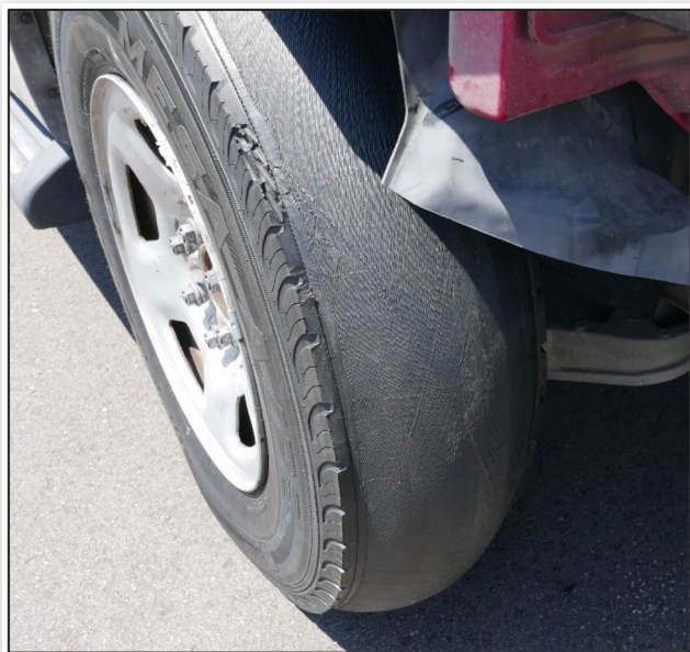
FIGURE 8 Tire with tread and top belt removed.
