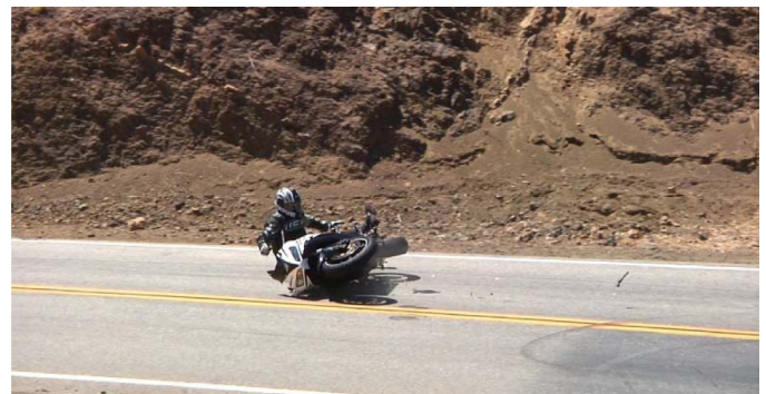
Figure 25. Rider Lands in a Seated Posture Facing Opposite His Initial Direction of Travel
