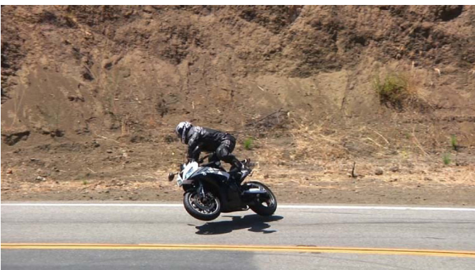
Figure 23. Lateral Forces from the Right Side Leading Sideslip Throw the Motorcycle into a Rightward Lean and the Rider is Launched Ahead of the Motorcycle
