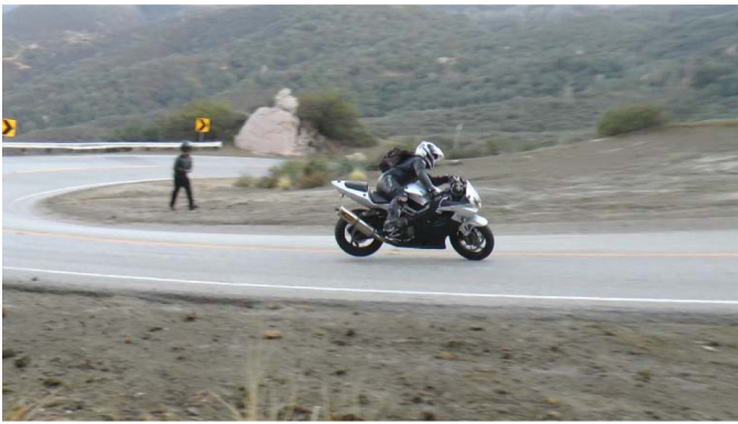
Figure 28. The Right Side Leading Yaw Ceases, the Motorcycle Yaws Clockwise and Rights Itself
