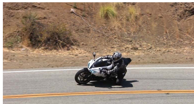
Figure 19. Right Side Leading Sideslip, Counter-Steer, and Tire Mark
