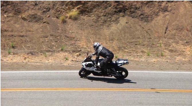
Figure 21. Rider Steers to the Left, Motorcycle Initially Continues to Towards a Leftward Lean/Fall, and a Left Leading Sideslip Develops
