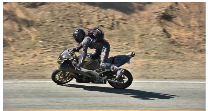
Figure 12. Rider Steers to the Left, Motorcycle Initially Continues to Towards a Leftward Lean/Fall, and a Left Leading Sideslip Develops
