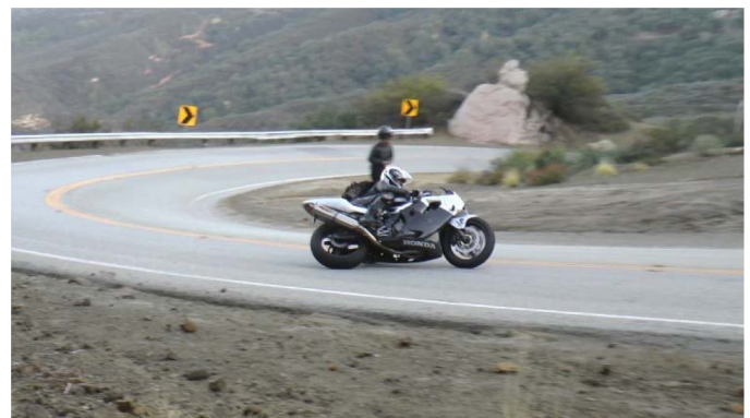
Figure 27. Right Side Leading Sideslip and Counter-Steer
