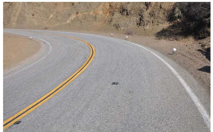
Figure 9. Examples of Tar Marks used for Reference Points in Video Analysis
