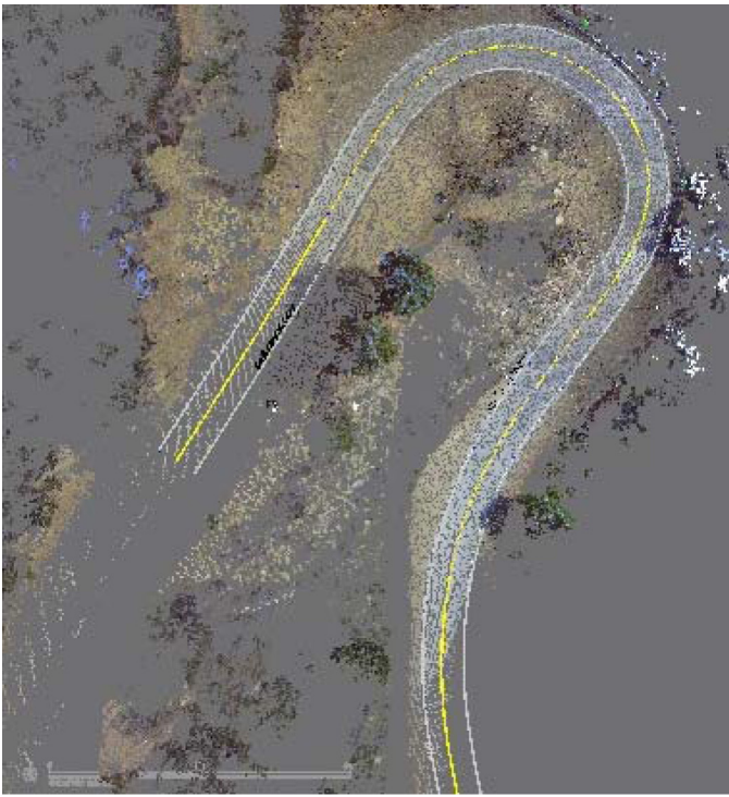
Figure 6. Survey and Scan Data of Edwards Corner Combined
