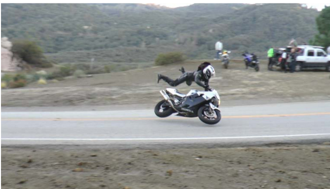
Figure 30. Left Side Leading High-Side Fall
